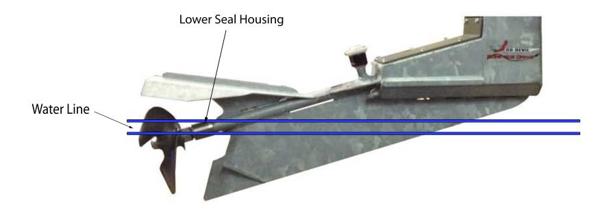
After getting on plane and to full throttle, take notice of the propeller depth. Trim up the motor until the water line is between the top and bottom of the lower seal housing and 1/3 of the prop will be above the water. A new motor and prop should run between 3400-3800 RPM when trimmed properly. This is where the motor produces it maximum horsepower.
