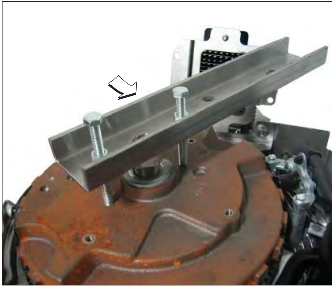
Figure 5-9 Install Flywheel Puller (Part No. 19621).
